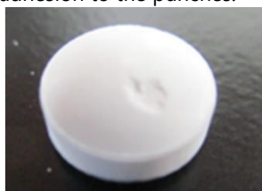
Fig. 3-a Tableting failure of the sample with PM
