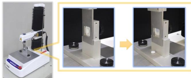
[Figure 1] Measurement of interfacial strength by Texture Analyzer
