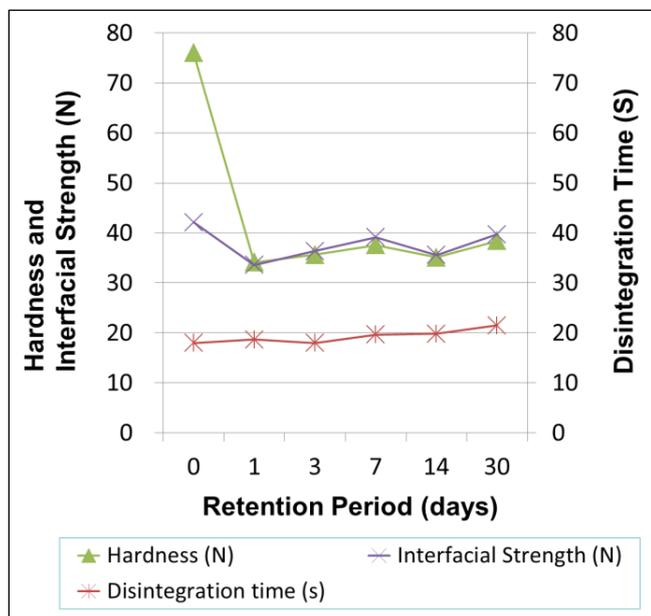
[Figure 3] Storage stability under unpackaged condition at 40°C/75%RH
