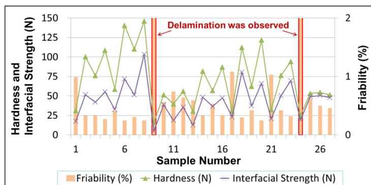
[Figure 5] Interfacial strength and friability of bilayer ODTs containing APIs
